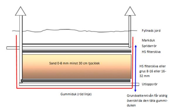
As a receiver and post-polishing, they have used HS ground bed of 1.2 m2 which is a very common package when installing.
