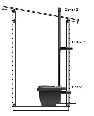
Please note that the ventilation works best if the pipe is pulled as straight up as possible. If you must make bends in the line, it may be wise to add a wind fan (accessory) to the end of the pipe to improve traction.
