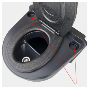
Next, you need to decide which side to run the ventilation pipe. There are ready-made places for the pipe to exit on both sides of the toilet seat. Once you've made your selection, cut a hole for the ventilation pipe on that side. A knife can be used for cutting, as the cutting seam is already thinned.
